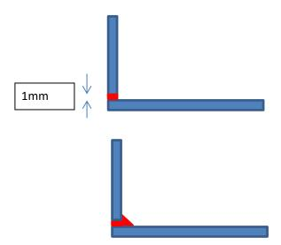
A triangular bead should be run on the internal face of the joint. The size of this bead is dependent on the capacity of the aquaria. This should be 2mm higher than the joint between the glass panels on small aquaria and 6mm higher than the joint on the largest aquaria
