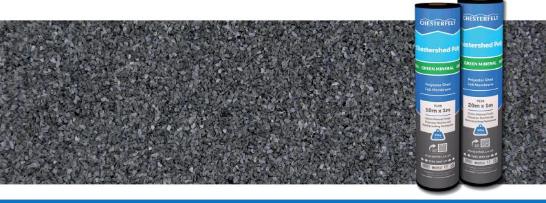
Chestershed Poly Mineral is a waterproof protection layer for use on portable type buildings with pitched roofs, such as sheds, stables, kennels and non-inhabited buildings. It features a polyester base which is saturated and coated in SBS modified bitumen and finished with light sand on the lower surface and green mineral granules on the upper surface
