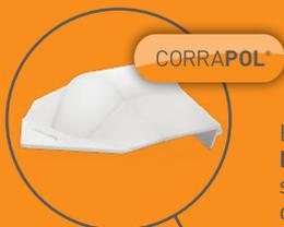
Fill small 2mm gap between the **CORRAPOL® Ridge End Cap** and the **Super Ridge Bar** with suitable sealant to create a waterproof seal on both sides of the roof.
