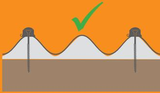
Fit **EITHER** roof nails **OR** screw cap fixings at **EVERY SECOND CORRUGATION PEAK** at each of the purlins, plus the top and bottom of the roof structure.
