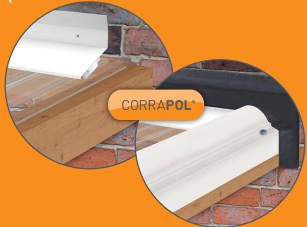
Cut off the Eaves Filler lugs at a **45° angle** to accommodate the curve on the **CORRAPOL® Side and Wall Flashing Bars**.
