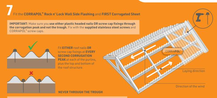
NOTE: It is advised to predrill an approx. 4mm pilot hole to accept the CORRAPOL® Flexi Cap screws. Use a HSS drill bit for this.
