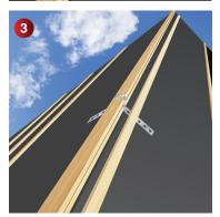
Install the top tiling batten as normal, leaving a 10mm air gap.
