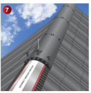
Insert the long and two short ratchet clips loosely into the middle and side slots respectively on the union. Lay the ridge tile on the ridge roll starting at the gable end or hip abutment, and slide the union into the open end. Slide the next ridge tile into the open end of the ridge union and press all three clips firmly in place. Secure the union with the screws provided, through the long ratchet clips. Any protruding end of the union can be snapped off or folded behind the union.
