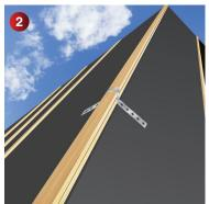
Build up the ridge batten using 25mm thick battens to the required height, usually two battens are sufficient for most profile tiles. Secure the battens in place using the stainless steel batten straps provided. Where Easy-Verge U is to be installed, the ridge batten must extend beyond the ridge by 30mm at each gable end.
