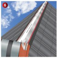
Remove the release paper from the butyl adhesive strip on the underside of each edge of the ridge roll, and firmly press onto the clean dry tile on both sides (avoid crushing the corrugations). Continue this process along the entire ridge line. Adhere the roll to the vertical surface of the dry verge unit at the gable end and at the hip abutment, overlap the roll across the hip rolls by 75mm, carefully sealing the butyl adhesive in place.
