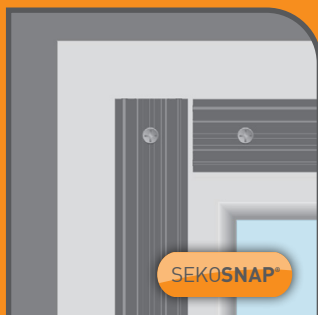
Square butt base plate and front top clip corner joint
