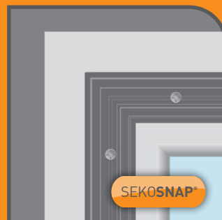
45 degree mitre base plate and front top clip corner joint
